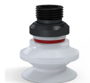
Variant reference: 91 31SLT 38D-2 • Color: Translucent • CE food certified • Matter: Silicone • Shore Hardness: SH60
